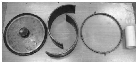
图 1 圆环形混凝土试块模具组成部件图 Fig.1 Diagram of mould formation for toroidal concrete block
