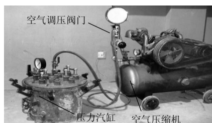
图 7 可控压力水头装置组装机 Fig.7 Assembly drawing of controlled water pressure device
