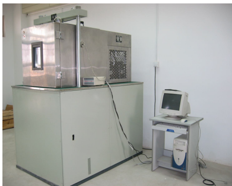
图 1 WDT-100 微机控制冻土试验机 Fig.1 WDT-100 PC-control tester for frozen soil experiments
