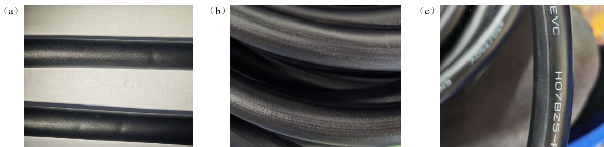
图 1 TPU 常见挤出质量问题: (a) 护套表面凹痕; (b) 护套表面磨砂效果频繁变化; (c) 护套表面磨砂颗粒度不均 Fig.1 Schematic diagram of common extrusion quality problems of TPU: (a) Sheath surface dents; (b) Frosted effect of the sheath surface changing frequently; (c) Uneven frosted particle size of the sheath surface
