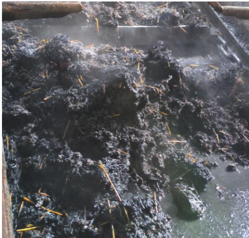
图 6 排渣口的生料与未燃尽焦炭 Fig. 6 Unburned straw and char at the outlet of grate
