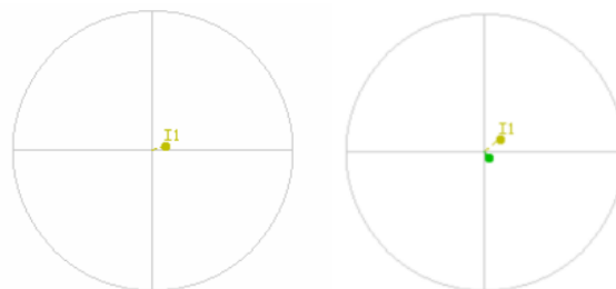
图 22 两相接地短路故障前后电流成分 Fig. 22 Current components before and after two-phase ground short circuit fault
