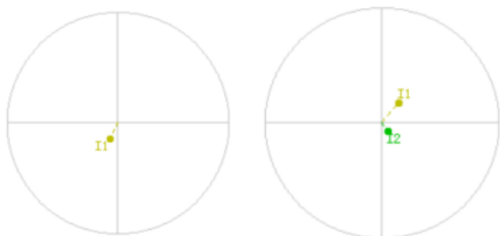
图 18 两相短路故障前后电流成分 Fig. 18 Current components before and after a two-phase short-circuit fault
