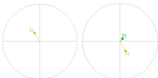
图 20 单相接地短路故障前后电流成分 Fig. 20 Current components before and after single-phase ground short circuit fault
