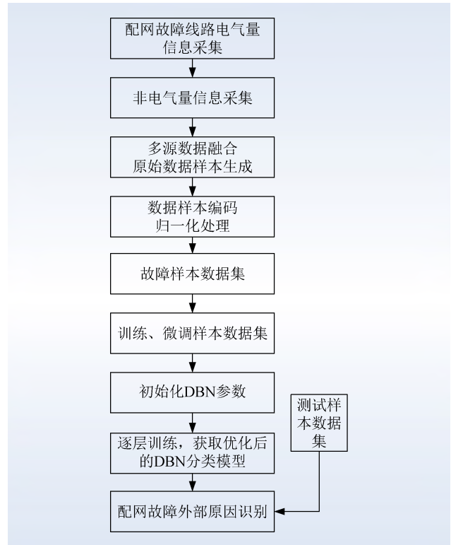
图 9 故障原因识别流程 Fig. 9 Process of fault cause identification
