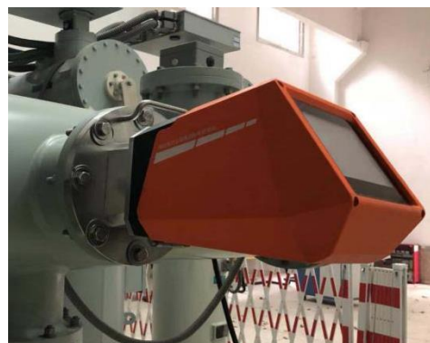
图 11 待测气体高压在线检测装置物理图 Fig 11. Physical diagram of high pressure on-line detection device of gas to be tested
