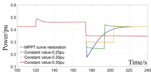
Fig. 4 Power waveforms of DFIG-VSG with constant-value restoration.
