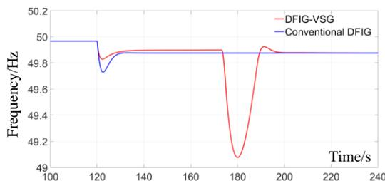
Fig. 9 Simulation results of wind turbine VSG with MPPT curve restoration
