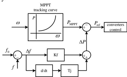
Fig. 1. Control diagram of wind turbine rotor inertia control.
