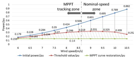
Fig. 5 Threshold value of constant power (Speed limit is set as 0.8pu).
