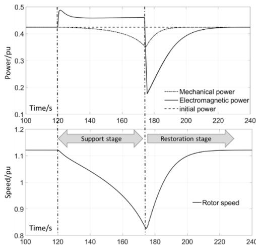
Fig. 2. Power and speed waveforms in frequency regulation with rotor inertia control.
