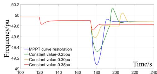
Fig. 10 Simulation results of wind turbine VSG with constant-value restoration.
