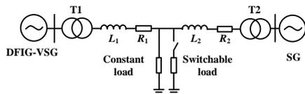
Fig. 8 Topology diagram of simulation system.
