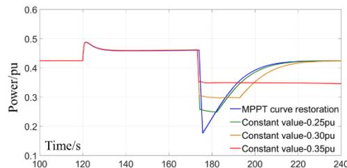
Fig. 7 Power waveforms of DFIG-VSG with comprehensive restoration
