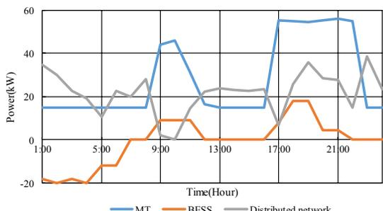
Figure 8. Optimal dispatching curves without considering load characteristic
