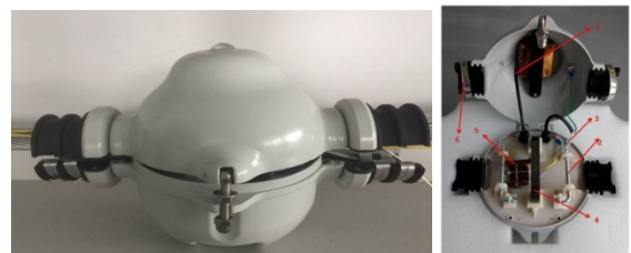
Fig. 2. The appearance and internal structure of five in one line rating ball
